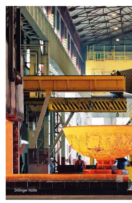
The process developed by Siempelkamp for plate forming allows for an optimum utilization of every single plate: The formed area directly reaches the chamfer of the subsequent weld.
