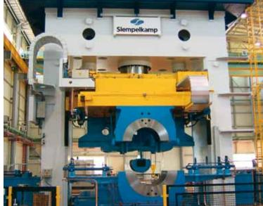
As leading manufacturer of individual presses for the production of large longitudinally welded pipes we offer the "A-U-O"-process in three forming stages. Due to the high production output of up to 30 pipes per hour this process stands out in comparison to other processes that are commercially available. For each of the three forming stages our customers get the optimum press including its auxiliary devices in the forming line.
