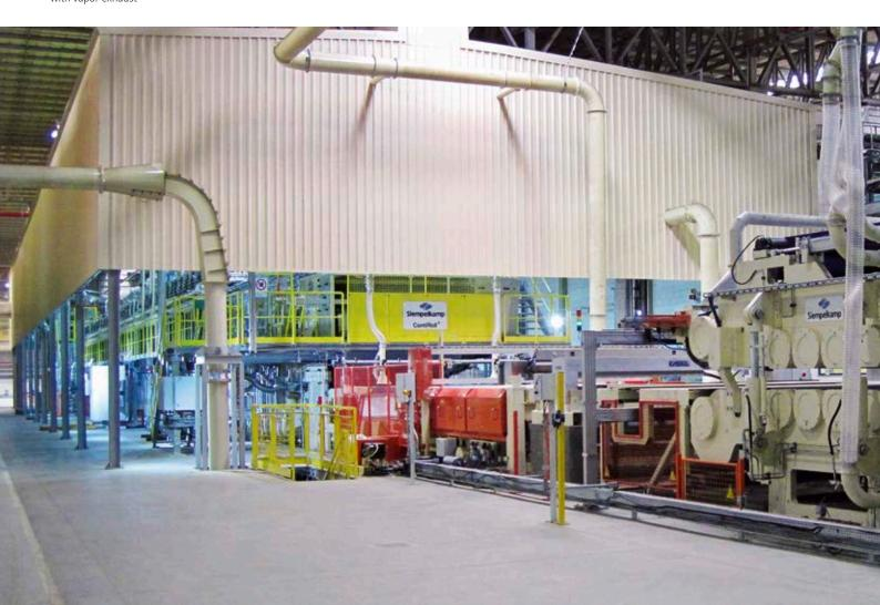
press and the company's second plant at the Curitibanos location. With the existing ContiRoll® line the customer has been manufacturing MDF. The new line will add particleboard to the product range.
