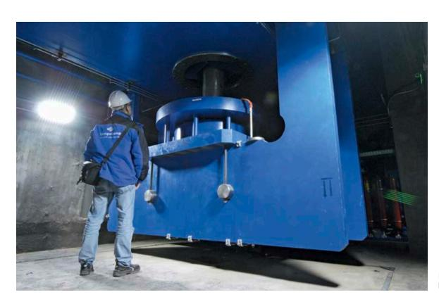
External ejector installed beneath the floor
