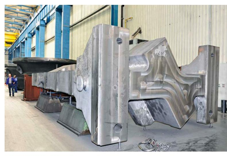
Press frame for a forging press in the machine shop
