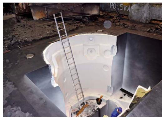
Pattern making for Adwen machine housing at the foundry
