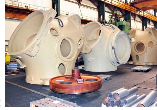
Rotor hub in the machining shop
