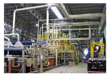
Forming line with prepress and vapor exhaust
