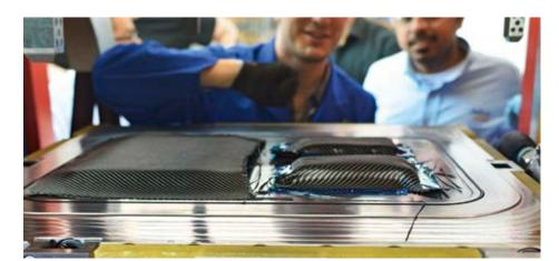
Lower press table with molds and preforms
