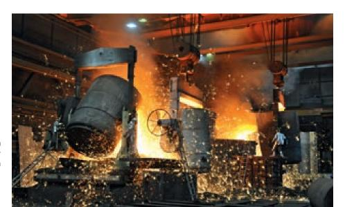
Record casting of a 283-ton upper beam for a press system
