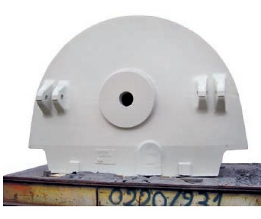
Cast component for a tile press
