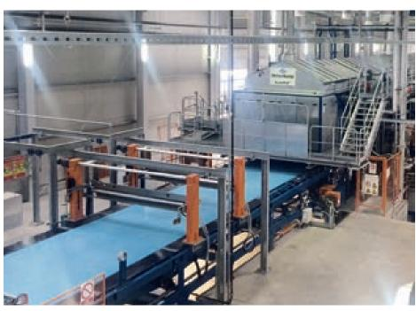
From left to right: the pre-press with trimming saw and press infeed
