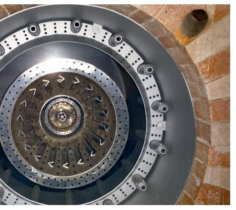
Büttner gas burner type BCB-G-35 with a capacity of 35 MW (120 MMBTU). The picture shows the gas nozzles and the air ring gap from inside the combustion chamber
