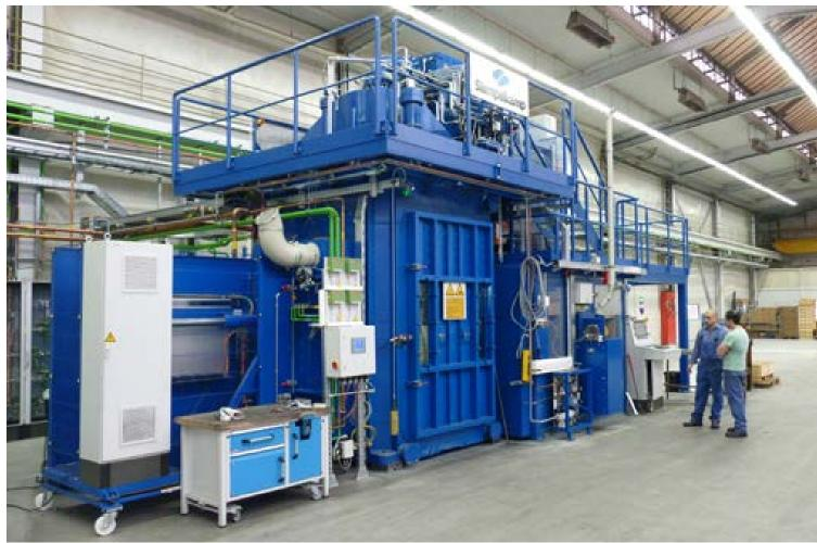
First of three isothermal forging cells for Leistritz
