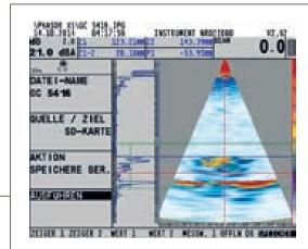
Direct comparison: conventional ultrasonic image (center) compared to a spatial phased array image (sector right)
