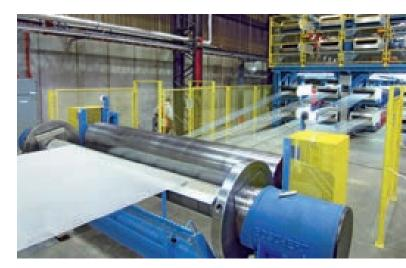
Individually controlled steel cord tension distribution system
