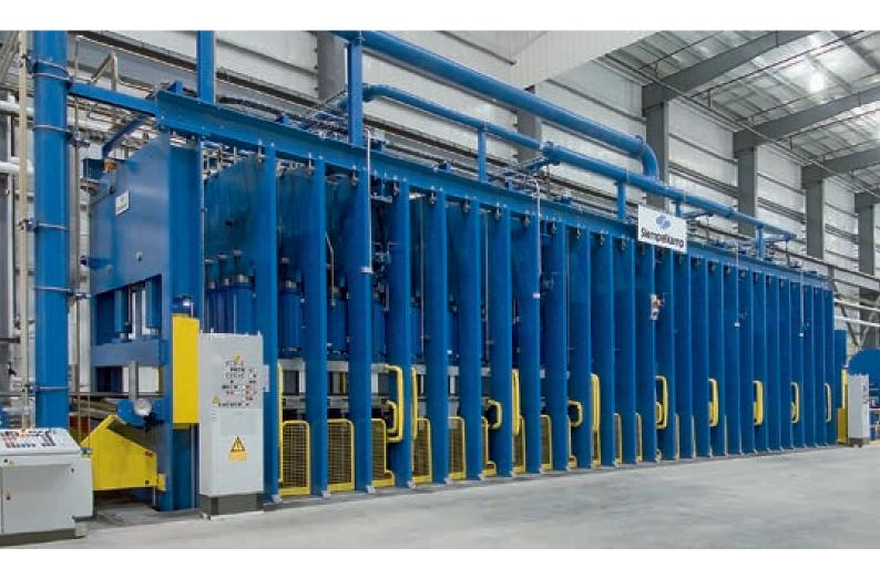
Siempelkamp presses and plants for the rubber industry are characterized by their long life cycles, high efficiency, and transparent process control. They are used for the production of flooring materials, rubber sheets and mats with smooth surfaces as well as conveyor belts.
