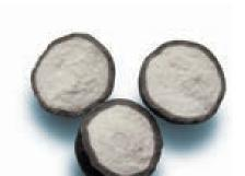
Cross-section through the catalyst material
