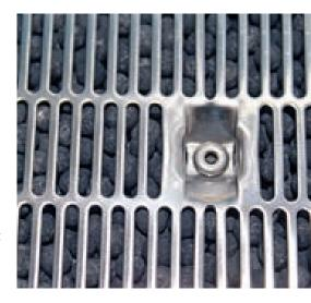
Catalyst material filled into a cartridge
