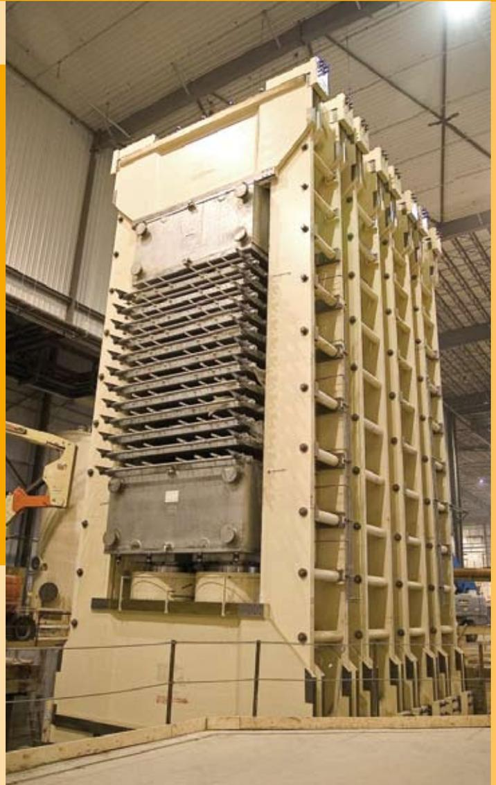
Canfor-LP, 12-daylight press during assembly
