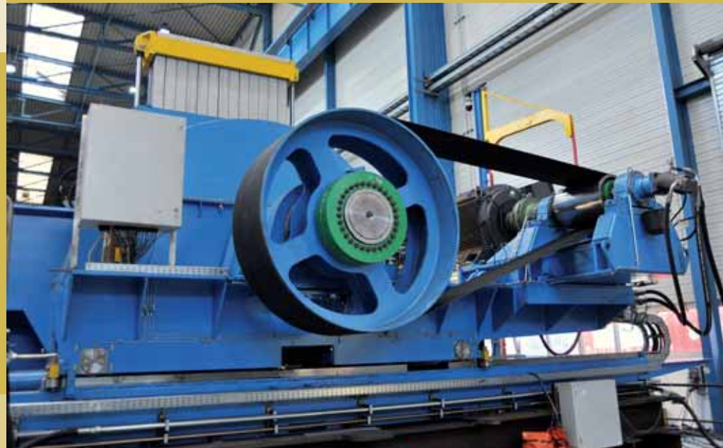
Impressive dimensions – strander from its main drive side
