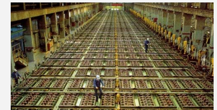
Fig. 5: Chlorine electrolysis with Hg contamination
