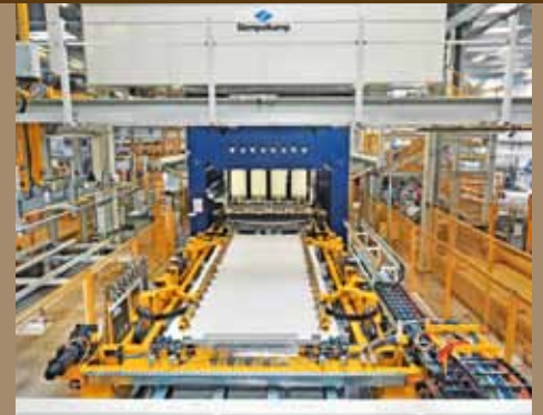
The finished panel is leaving the press
