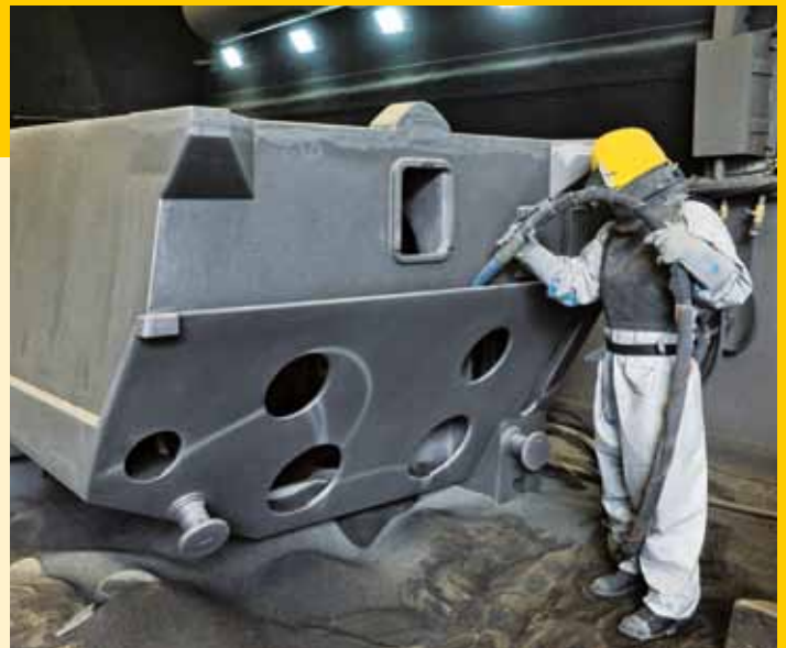
"Fine-tuning" of the machine bed in the fettling shop
