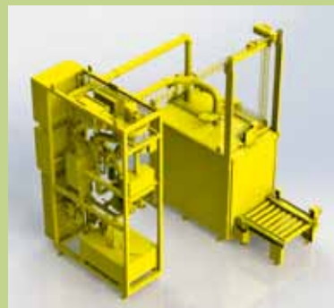
3-D model of the C2 facility package (waste treatment plant) for Hainan NPP: left – drying, sorting and compacting system, right – drum drying plant
