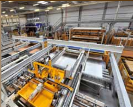
Placing of the board on the backing
