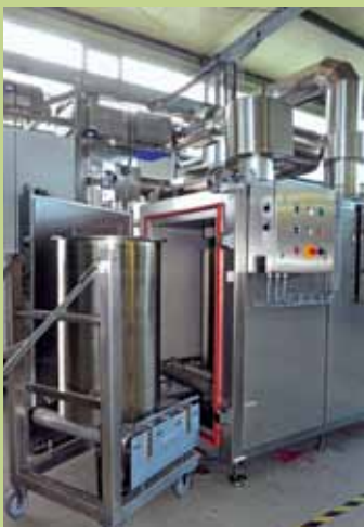
Trolley and drum conveyor of the drying chamber
