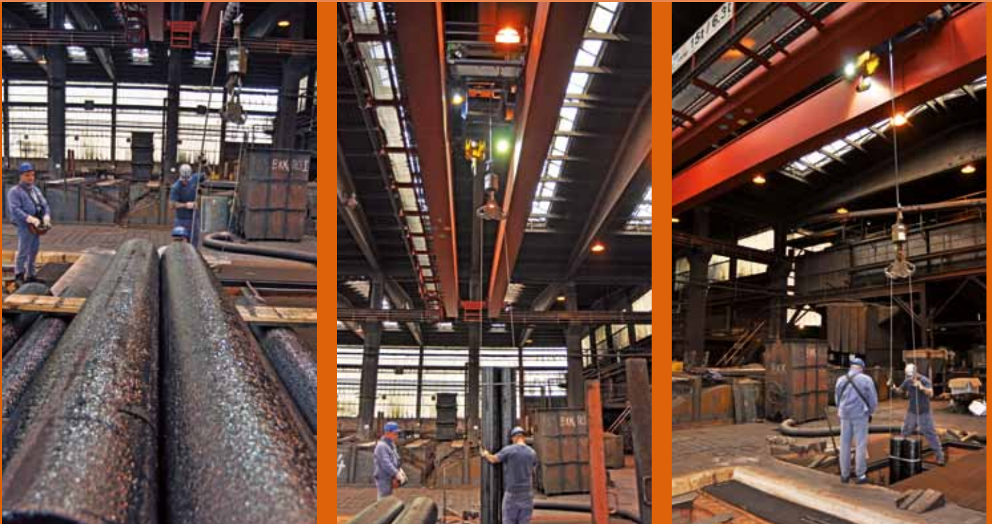
Transport and assembly of the graphite bar blanks into ring kiln chambers
