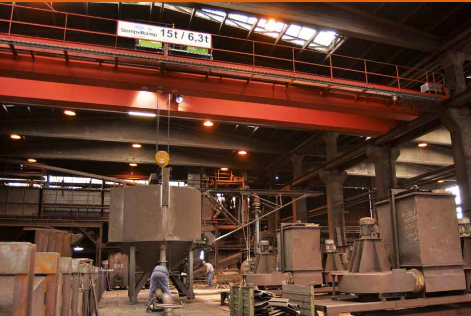
Transport of a suction device by the Siempelkamp crane system
