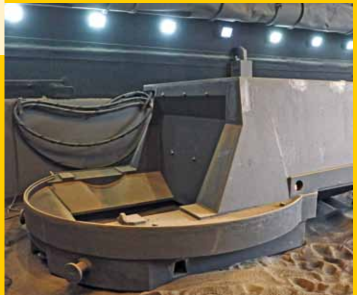
"Fine-tuning" of the machine bed in the fettling shop
