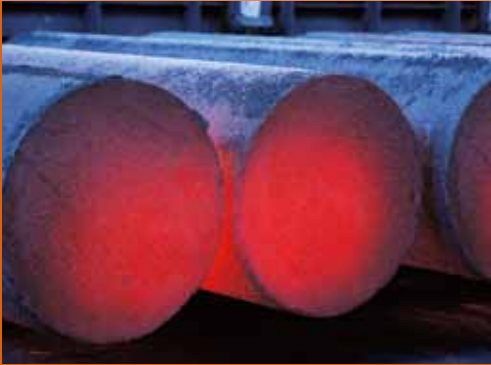
Glowing graphite electrodes after graphitization (photo: 2010 ©SGL Group)
