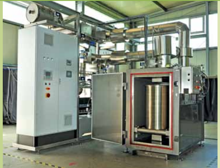
Two-drum drying plant for Qinshan nuclear power plant, phase II
