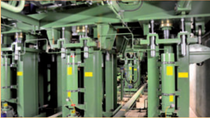
The hydraulic damping of the roller tables
