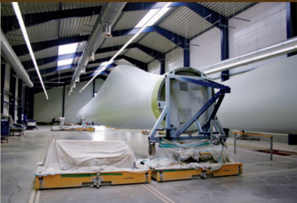
The hub of the 44 m long blade has a diameter measuring almost 2 m
