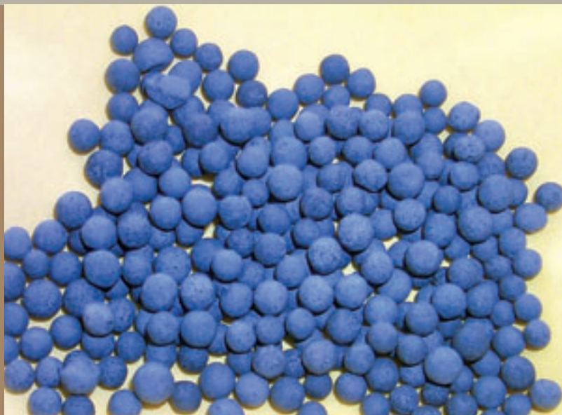
Palladium-coated catalyst material
