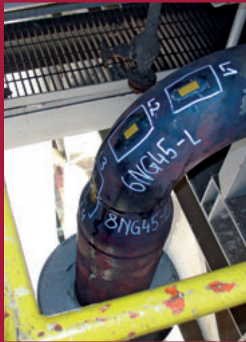
Replica testing of an elbow pipe
