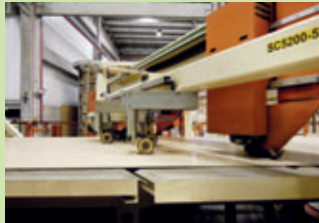
Diagonal saw at press outfeed area
