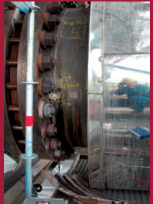
Replica testing of the welded seam of a flange
