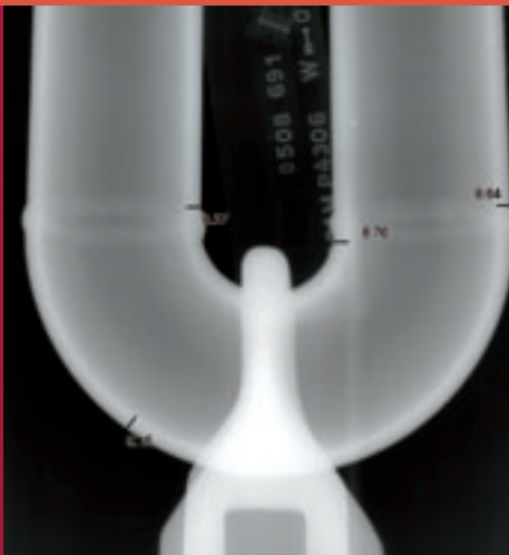
Radiographic inspection of a pipe elbow
