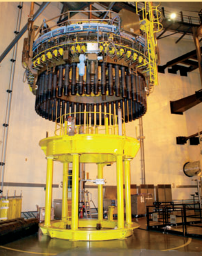
Castor® cask body during mechanical machining
