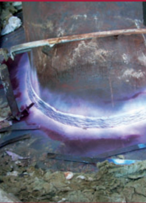
Surface crack testing of a welded seam
