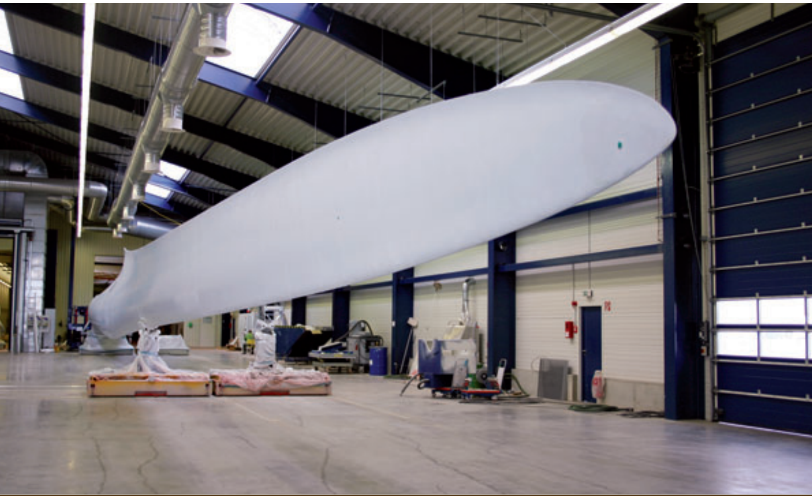
On the RoundTrack®, the parts are automatically driven through the paint shop
