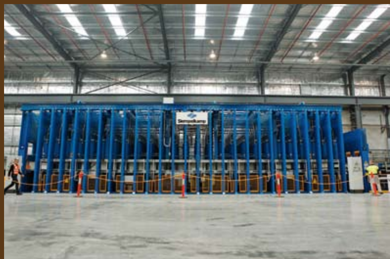
Vulcanizing press: 3,200 mm x 18,480 mm; 156 cylinders; 25,000 t
