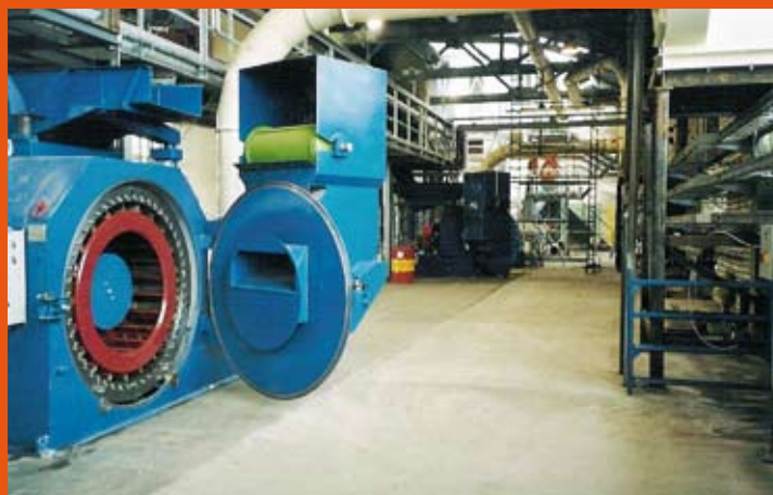
Left: Knife-ring flaker Right: Rotor
