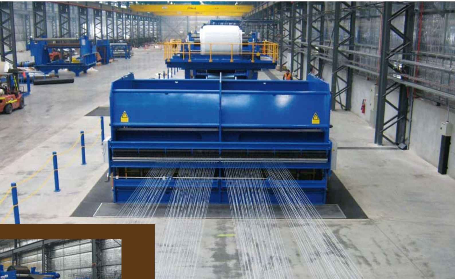
From the creel to the infeed of the cable tensioning system
