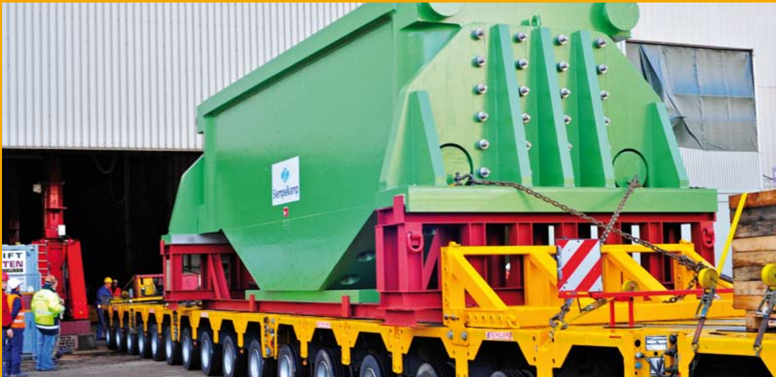
Delivery of the lower bolster to the construction site
