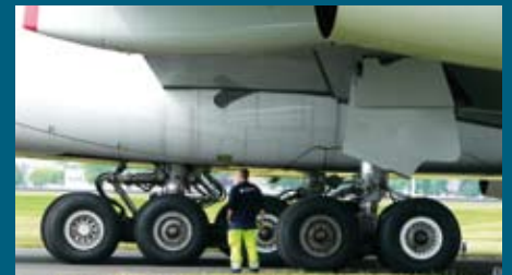
The chassis of an Airbus A 380: Many components are forgings made of titanium
