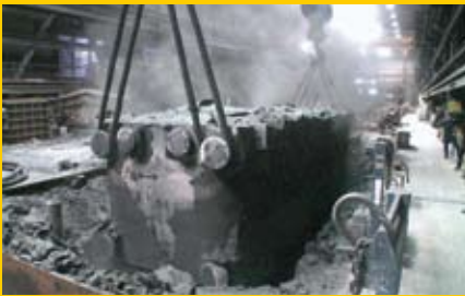
Lifting of the finished part
