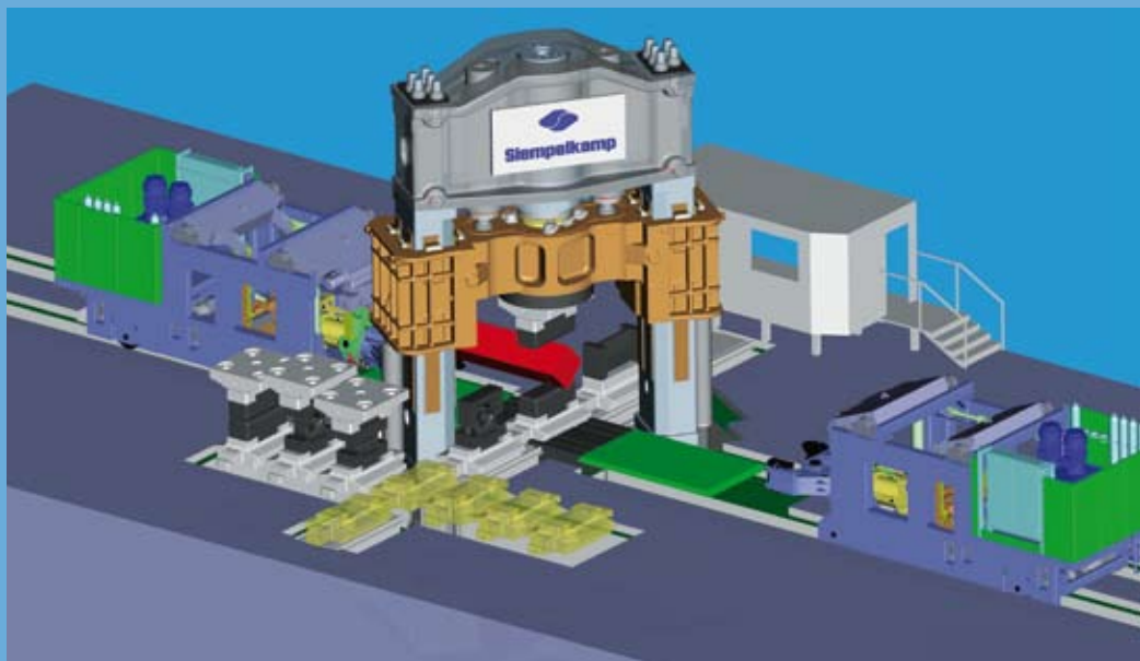
Siempelkamp supplies the new open-die forging press including hydraulics, die change system and two manipulators which position workpieces precisely for forging
