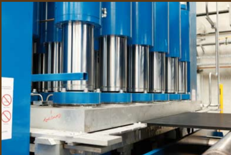
Press infeed with 6 cylinders arranged along the width direction
