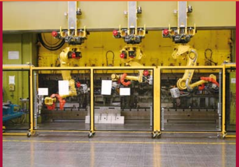
The suspended frame attachment with three robots on each side of the side member press
