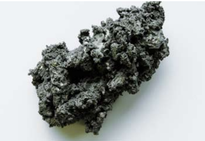
Titanium sponge is extremely porous and has to be compacted
