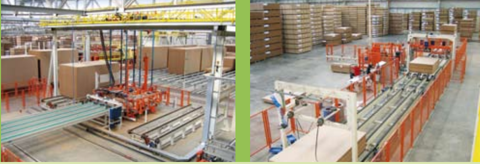
Left: Stacking and packing line Bottom: Duratex 77-m cut-to-size system and cooling and stacking line
